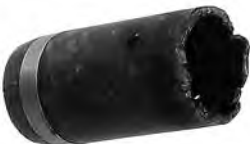
Sheaffer cap with advanced crazing.
